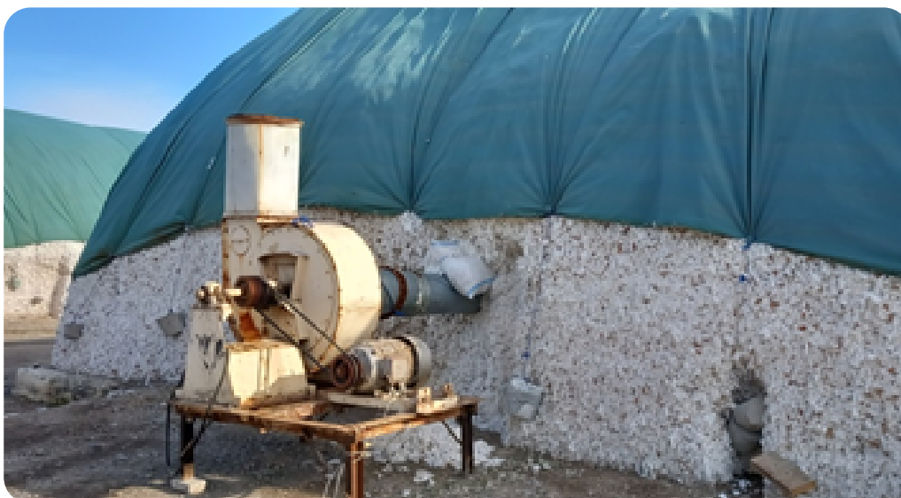
Equipment for extracting moist air from cotton bales, 2022
